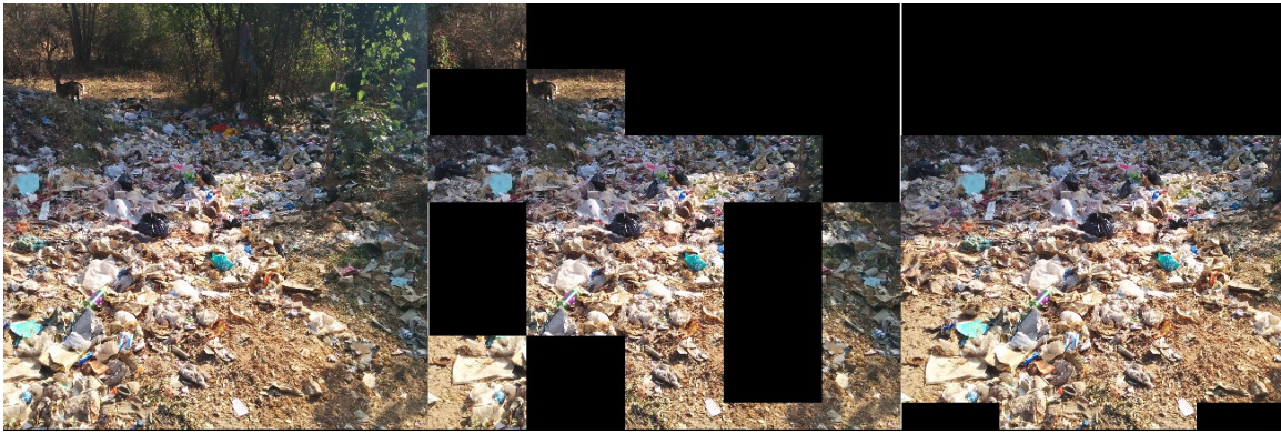
Figure 3: Comparison of results of segmentation using sliding windows with edge thresholding vs fully connected neural network. Left is original image. Center is segmentation result using edge thresholding. Right is segmentation result using fully connected neural network.
