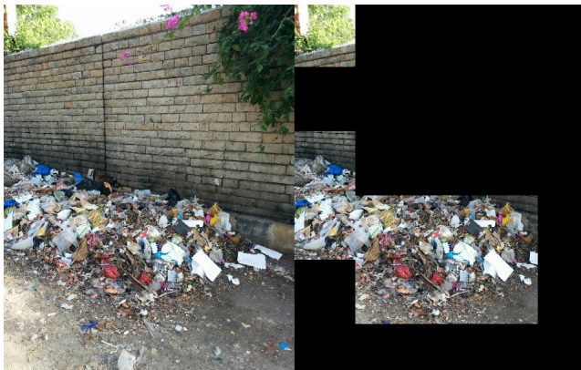
Figure 2: Results of segmentation using sliding window and edge thresholding approach. Left image is original image. Right is image after segmentation.
